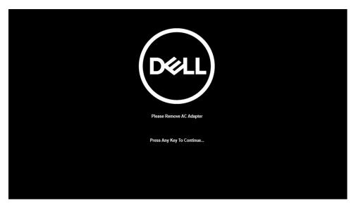
5. When the ready-to-proceed message appears on the screen, press any key to proceed. The system emits three short beeps and shuts down immediately.
