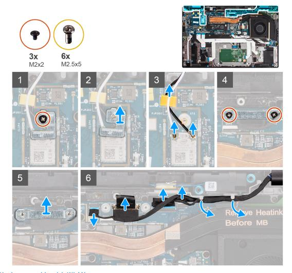
Figure 2. Display assembly with WLAN antenna
