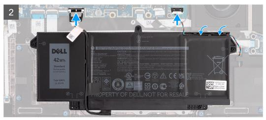
NOTE: If the battery is disconnected from system board, there is delay during computer boot as the computer undergoes RTC reset.
