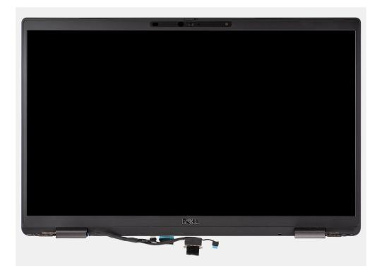
Figure 1. Display assembly without antennae cables
