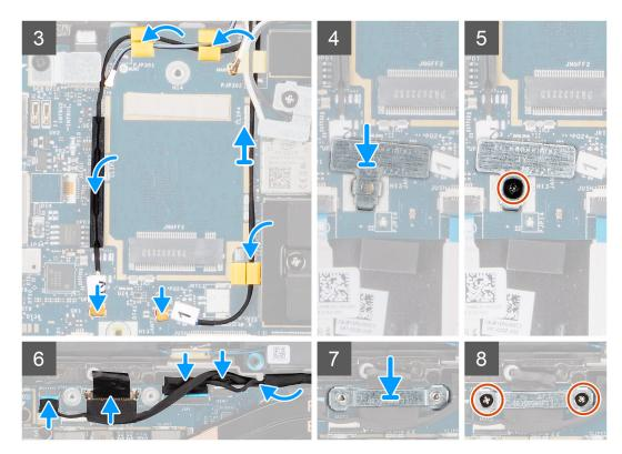
Figure 7. Display assembly with WLAN and WWAN antenna cables
