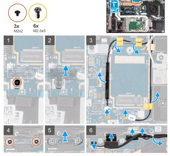
Figure 3. Display assembly with WLAN and WWAN antenna
