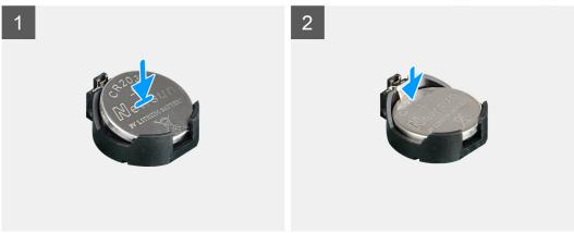
Insert the coin-cell battery into the socket with the positive side (+) labeled facing up and snap the battery in the socket.
