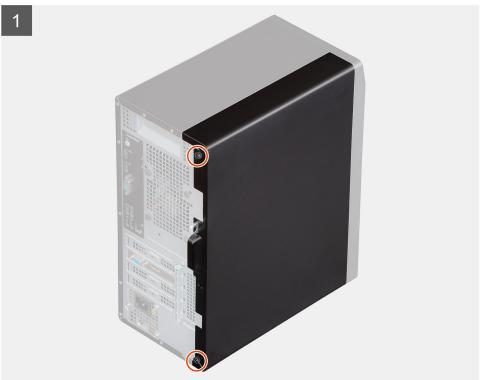
2. Using the tab on the right-side cover, slide back and lift the right-side cover off the chassis.
