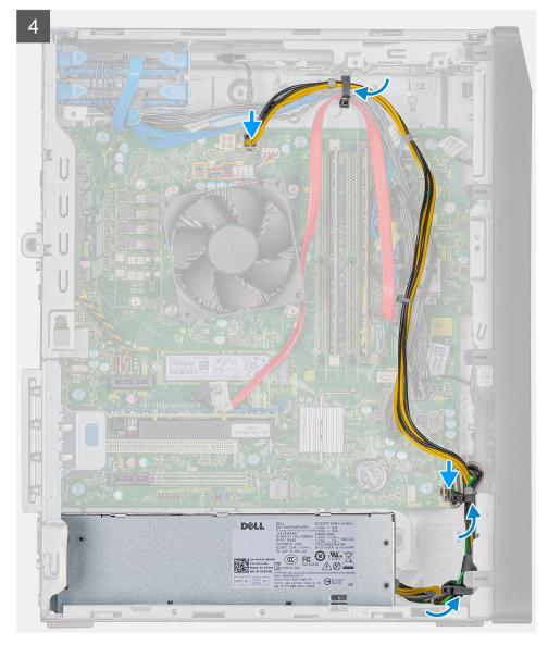
Installing power-supply unit with dual connector.
