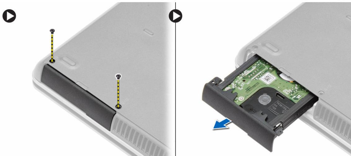
4. Remove the screw that secures the hard-drive caddy to the hard drive. Remove the hard-drive caddy from the hard drive.
