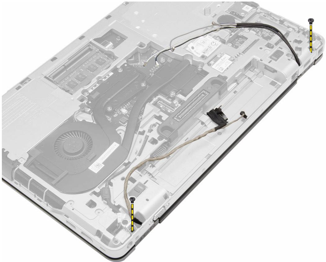
6. Remove the display assembly from the computer.
