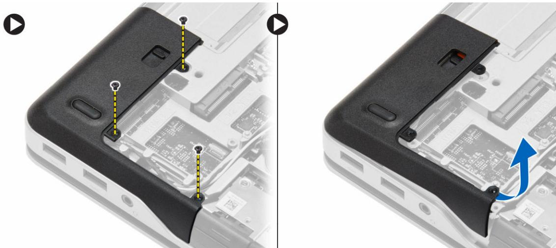
5. Remove the screws that secure the right base-corner cover, lift and remove it from the computer.
