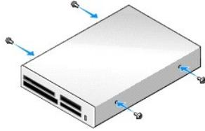
3. Align the shoulder screws on the media card reader with the shoulder screw slots, and gently slide it into the bay until it clicks into place.
