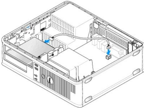
5. Align the shoulder screws with the screw guides, and slide the media card reader into the bay until it clicks into place.
