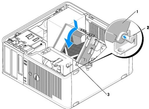
1 | heat sink assembly | 2 | heat-sink assembly bracket | 3 | captive screw housing (2)
