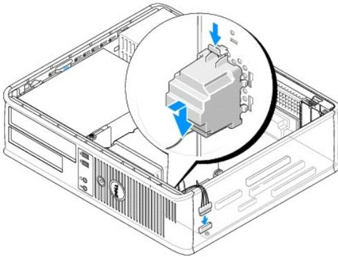
4. Connect the cables to the system board.
