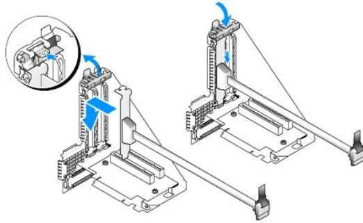
5. Plug the free end of the eSATA cable into the eSATA connector on the system board.
