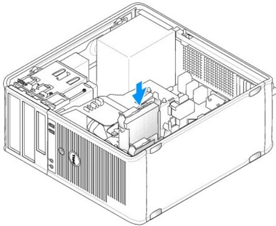
6. Carefully slide the hard drive into the drive bay until it clicks into place.
