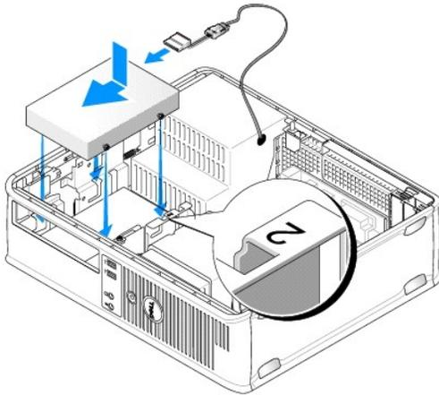
10. Locate an unused SATA connector on the system board and attach a data cable from the second hard drive to the SATA connector.
