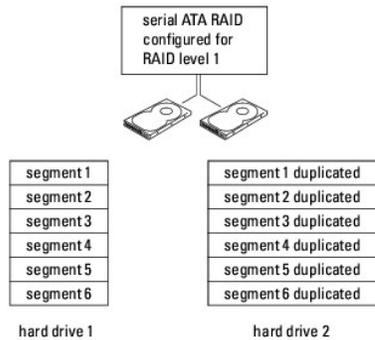
If a drive failure occurs, subsequent read and write operations are directed to the surviving drive. A replacement drive can then be rebuilt using the data from the surviving drive.
