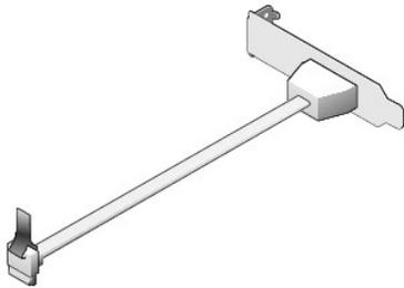
4. Plug the free end of the eSATA cable into the eSATA connector on the system board.
