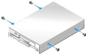
3. Align the shoulder screws on the floppy drive with the shoulder screw slots, and gently slide it into the bay until it clicks into place.
