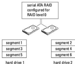
Another advantage of a RAID level 0 configuration is that it utilizes the full storage capacities of the drives. For example, two 120-GB hard drives combine to provide 240 GB of hard drive space on which to store data.
