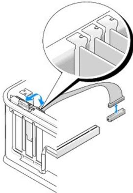
5. Ease the PS/2 serial-port adapter bracket out of its retention slot.
