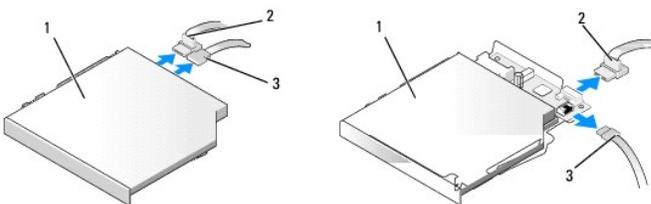
1 optical drive 2 data cable 3 power cable
