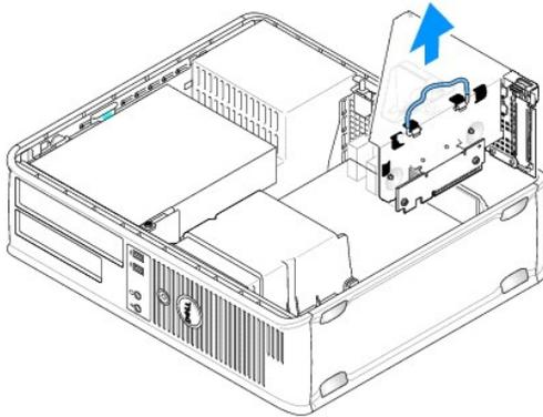
3. Press the blue release tab to remove the filler panel for the card slot you are using for the eSATA connector.
