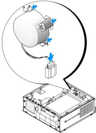
4. Connect the cables to the system board.
