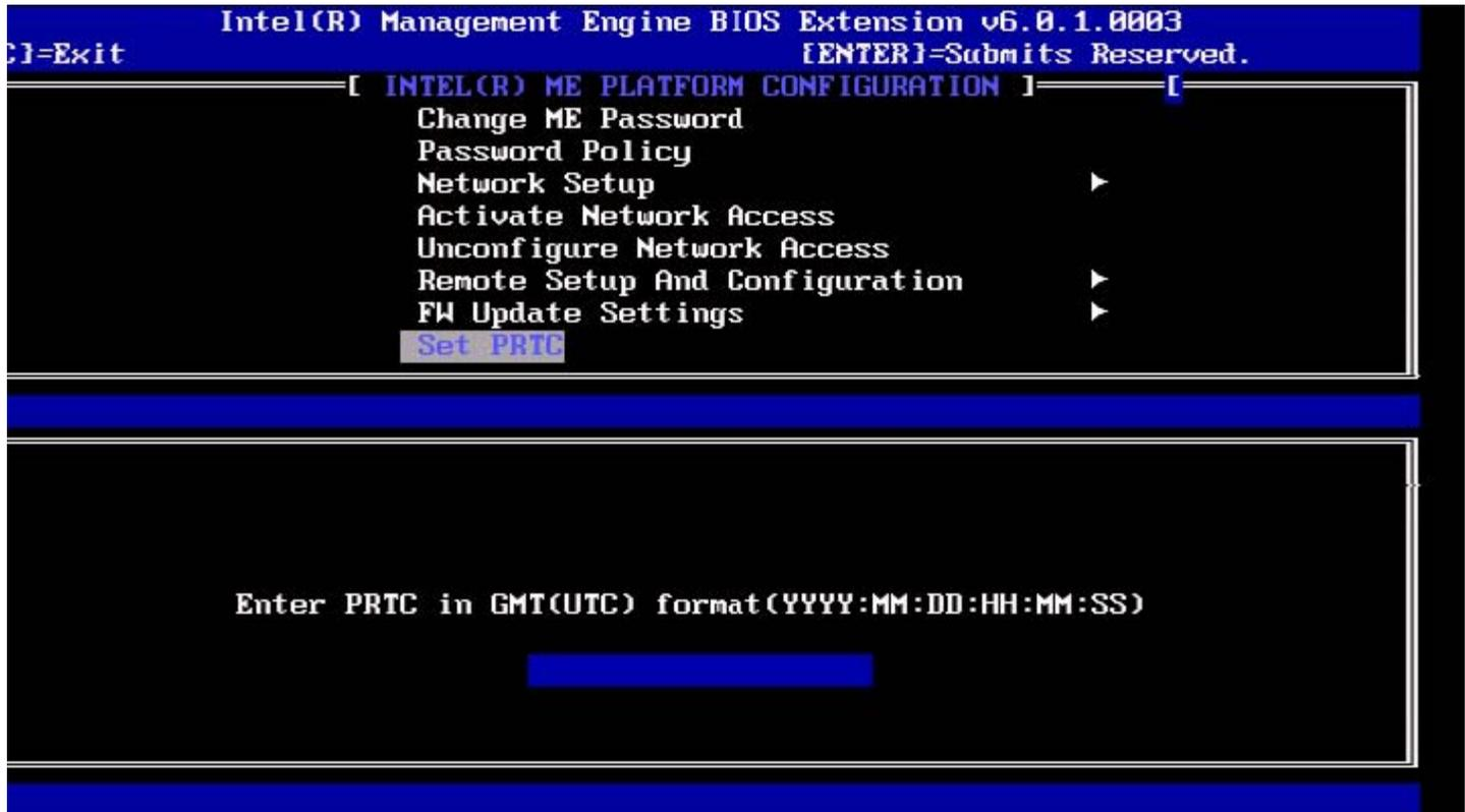
Valid date range: 1/1/2004 – 1/4/2021. Setting the PRTC value is used for virtually maintaining PRTC during the power-off (G3) state.
