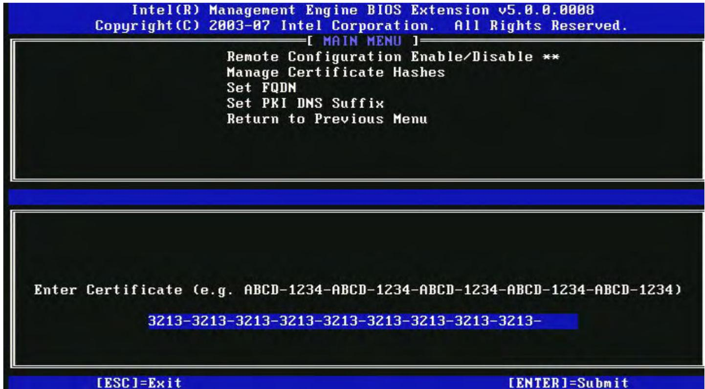
The Certificate hash value is a hexadecimal number (for SHA-1 it is 20 bytes for SHA-2 it is 32 bytes). If the value is not entered in the correct format, the message "Invalid Hash Certificate Entered - Try Again" is displayed. When you press
