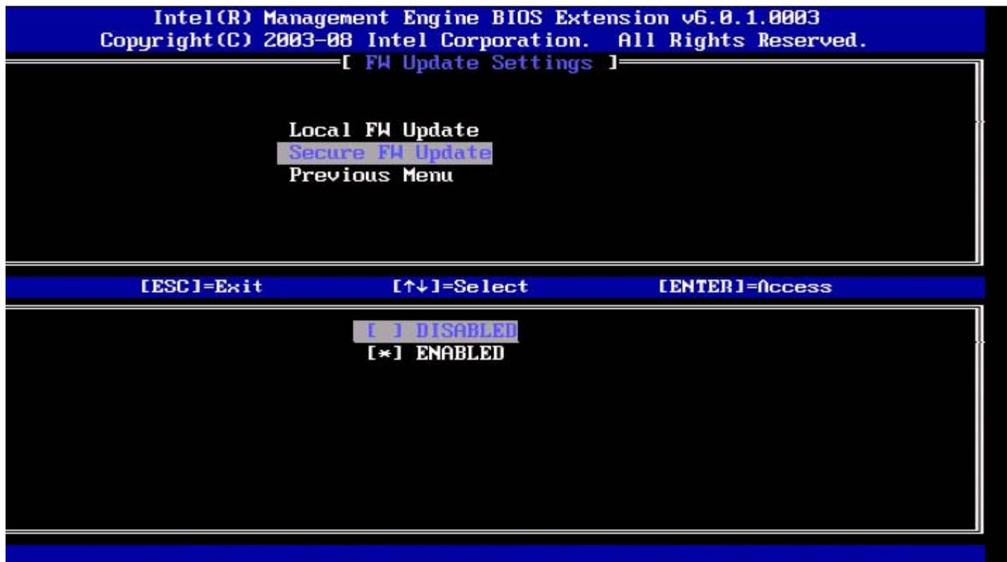
This option allows the user to enable or disable secure firmware updates. The Secure Firmware Update function requires an administrator user name and password. If the administrator user name and password are not supplied, the firmware cannot be updated.
