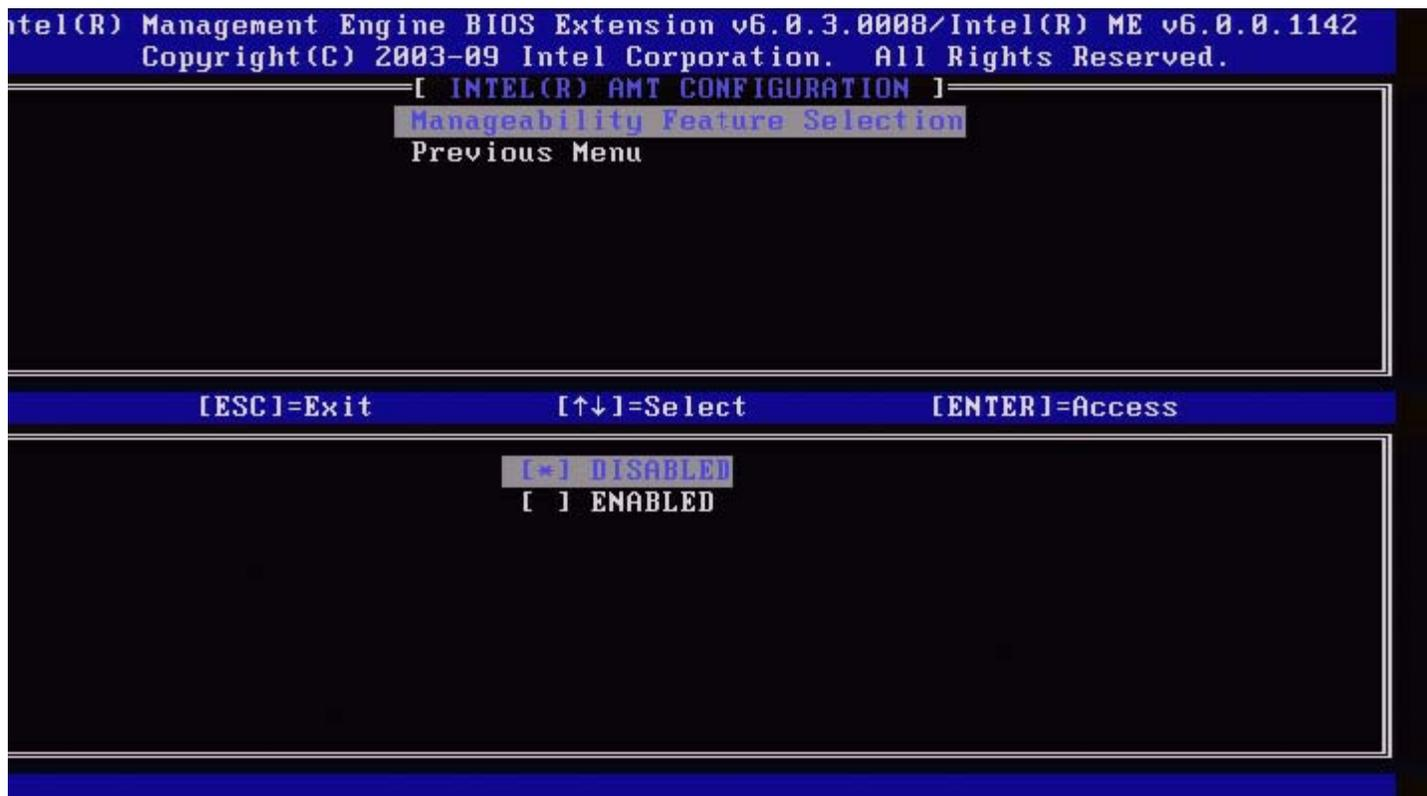
When the Manageability Feature Selection is enabled, the Intel ME manageability feature menu will be shown. Leaving it disabled means that manageability will not be enabled.
