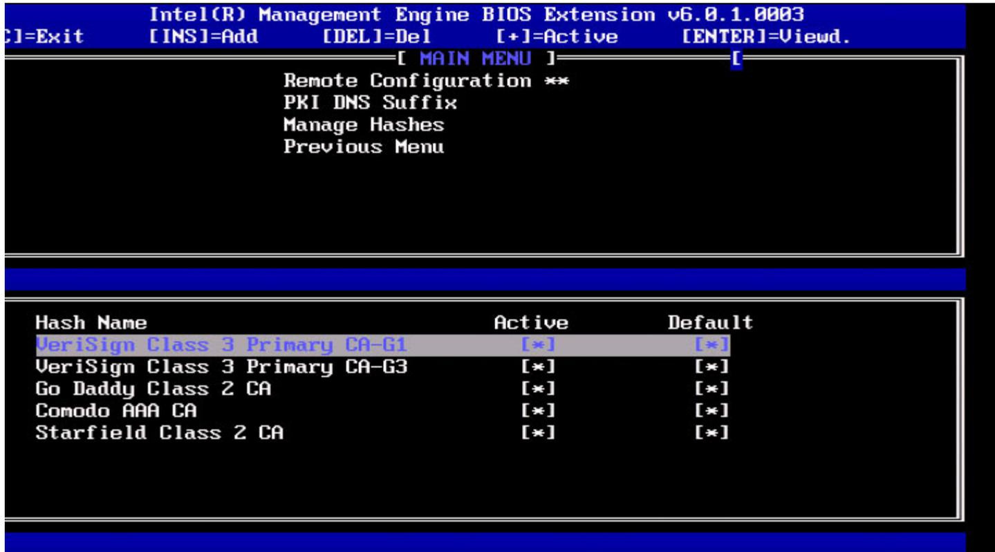
Selecting this option will enumerate the hashes in the system and display the Hash Name and the active and default state. If the system does not contain any hashes yet, Intel MEBx will display the following screen.
