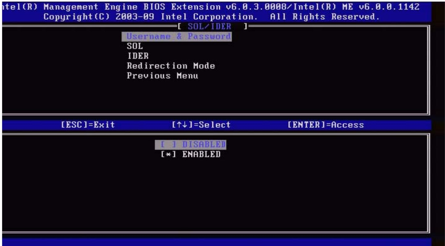
This option provides the user authentication for SOL/IDER session. If Kerberos\* is used, this option should be set to DISABLED. The user authentication is handled through Kerberos. If Kerberos is not used, the IT administrator has the choice to enable or disable user authentication on SOL/IDER session.
