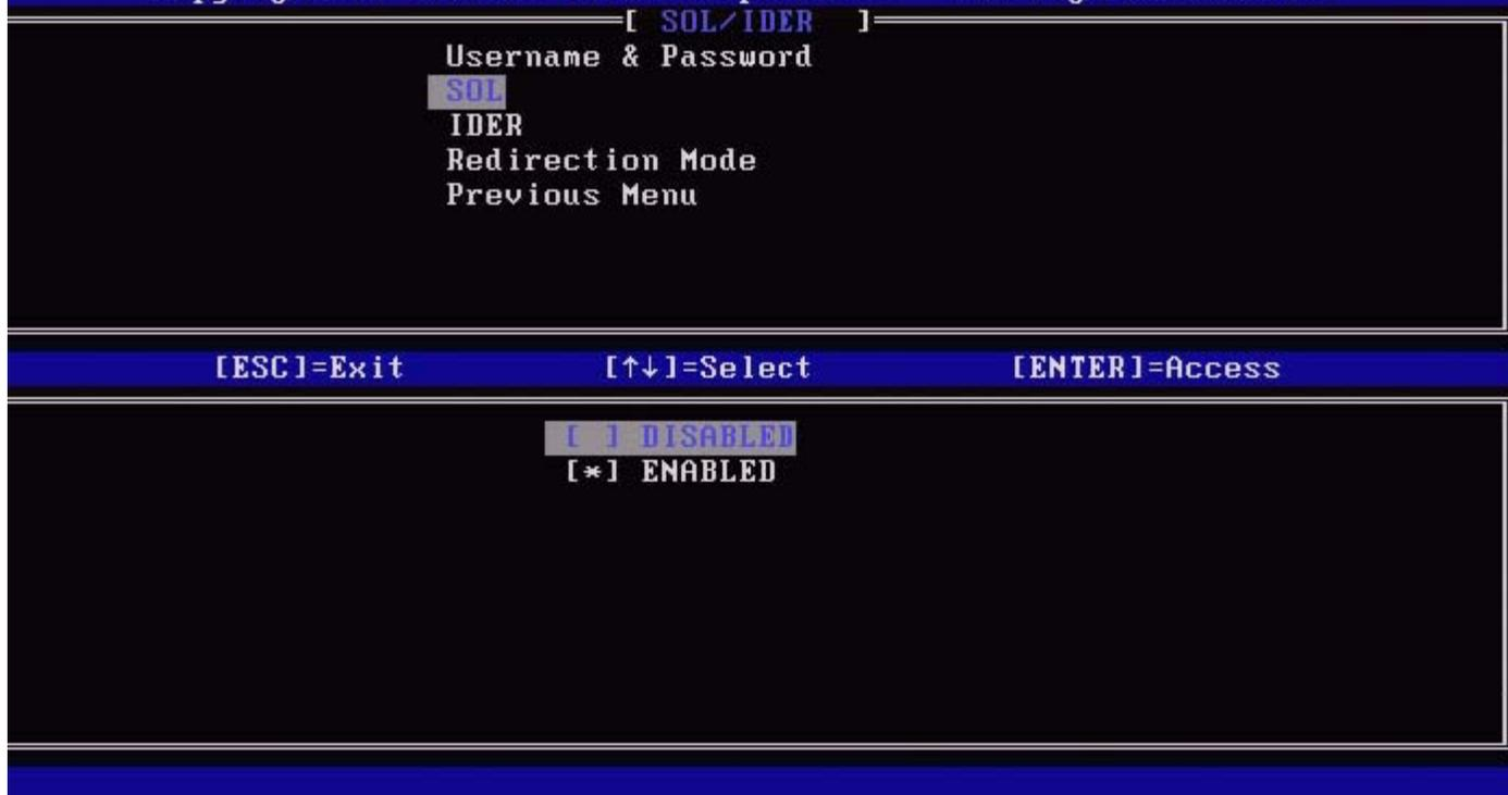
SOL allows the console input/output of an Intel AMT-managed client to be redirected to a management server console (if the client system supports SOL). If the system does not support SOL, this value cannot enable it.
