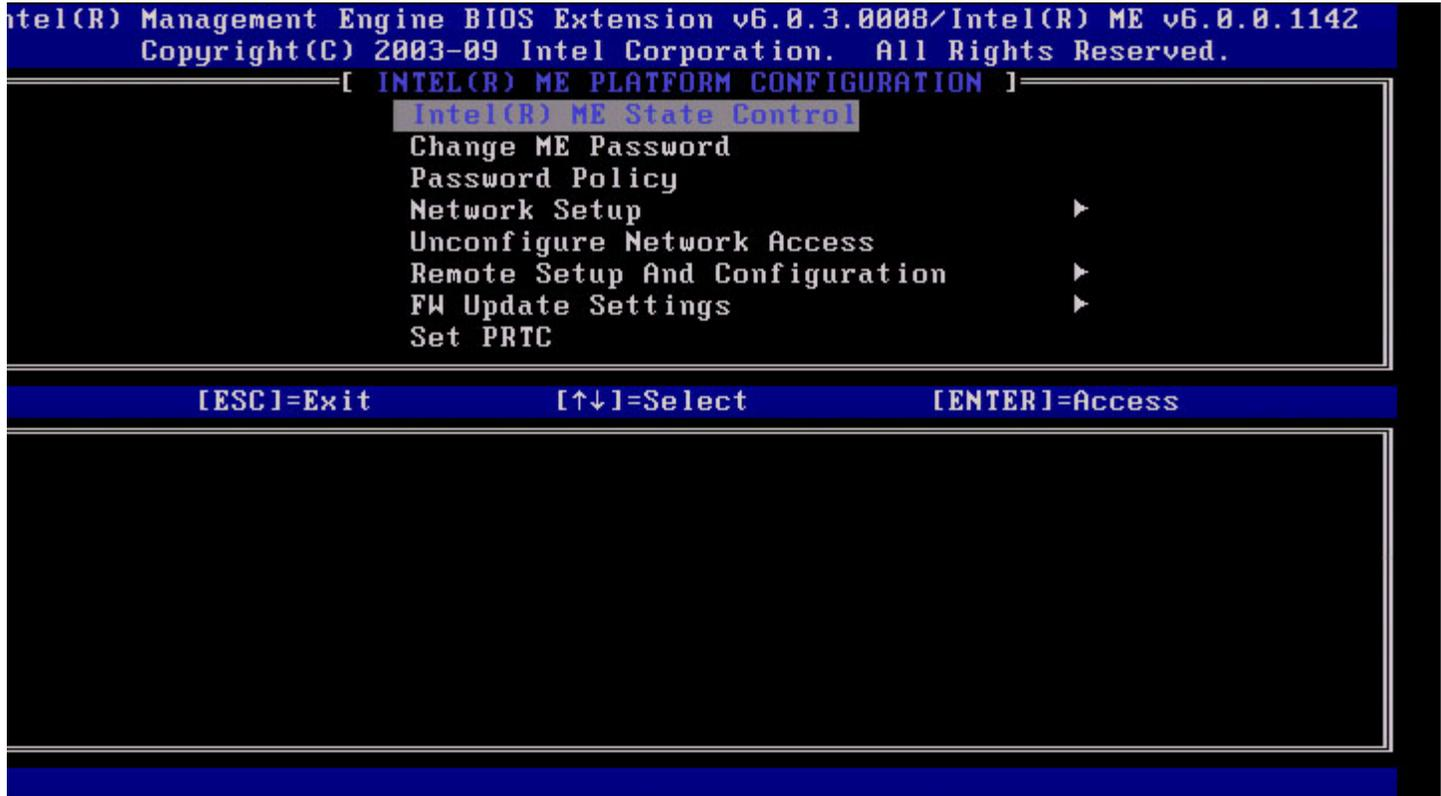
The Intel ME State Control option (**enable/disable**) provides the ability to disable the Intel ME for debugging purposes. Disabling the Intel ME through the MEBx prevents the Intel ME code from executing. This allows an IT technician to eliminate the Intel ME as the potential problem.
