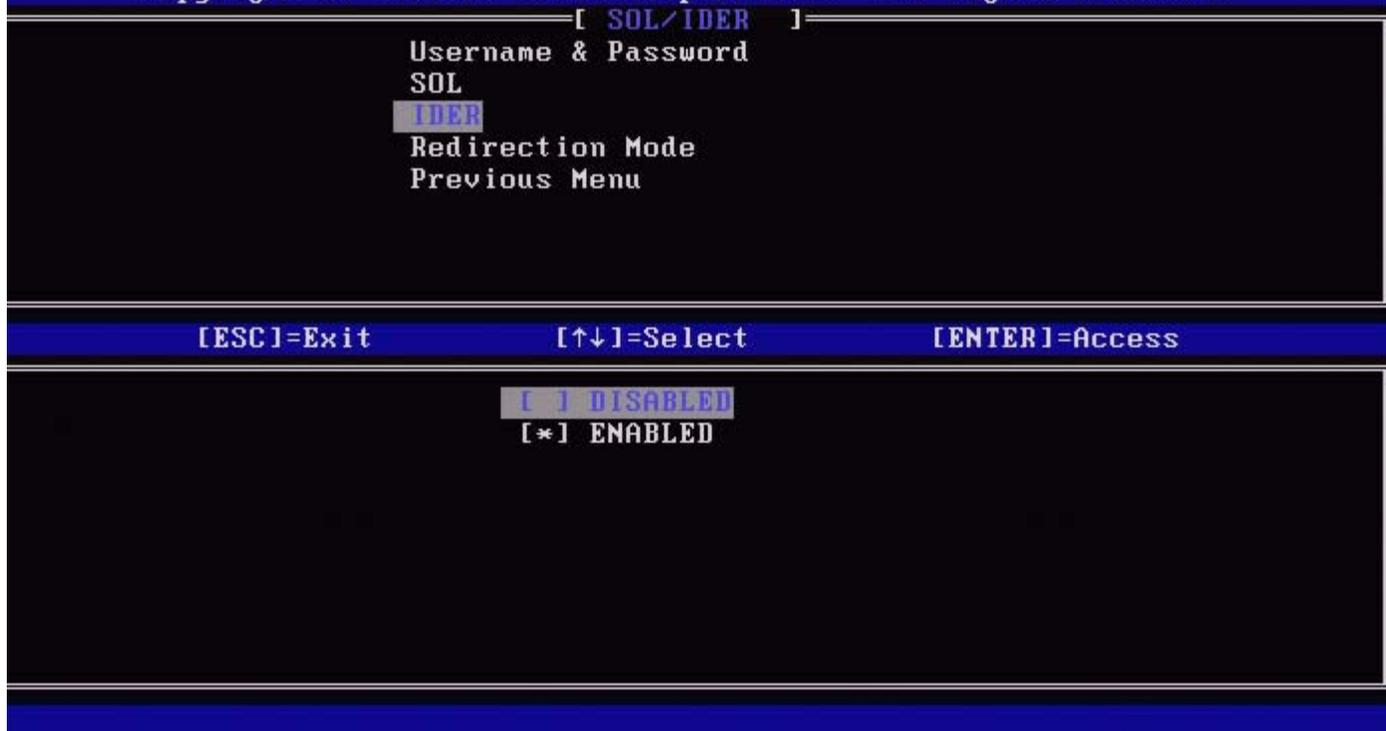
IDE-R allows an Intel AMT-managed client to be booted by a management console from a remote disk image. If the client system does not support IDE-R, this value cannot enable it.
