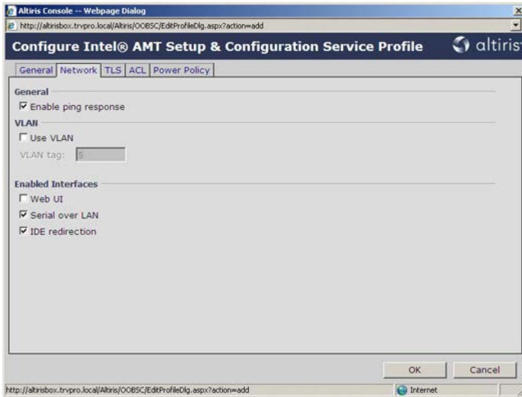
The screenshot shows the 'Configure Intel® AMT Setup & Configuration Service Profile' dialog box in the 'Network' tab. The 'General' section has 'Enable ping response' checked. The 'VLAN' section has 'Use VLAN' unchecked and 'VLAN tag' set to 5. The 'Enabled Interfaces' section has 'Web UI' unchecked, 'Serial over LAN' checked, and 'IDE redirection' checked. The dialog has 'OK' and 'Cancel' buttons at the bottom right.
