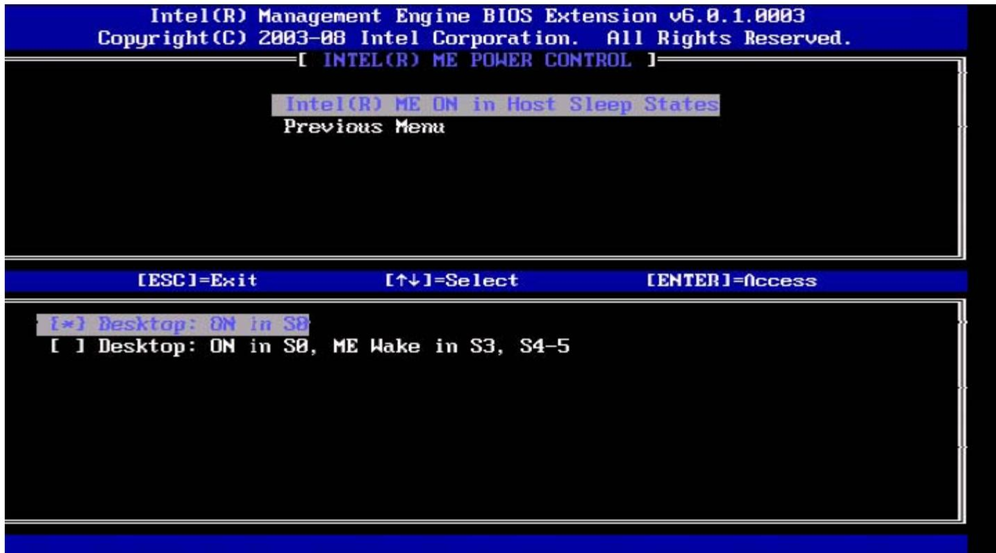
The selected power package determines when the Intel ME is turned ON. The default power package can be modified by using FITC or by FPT.
