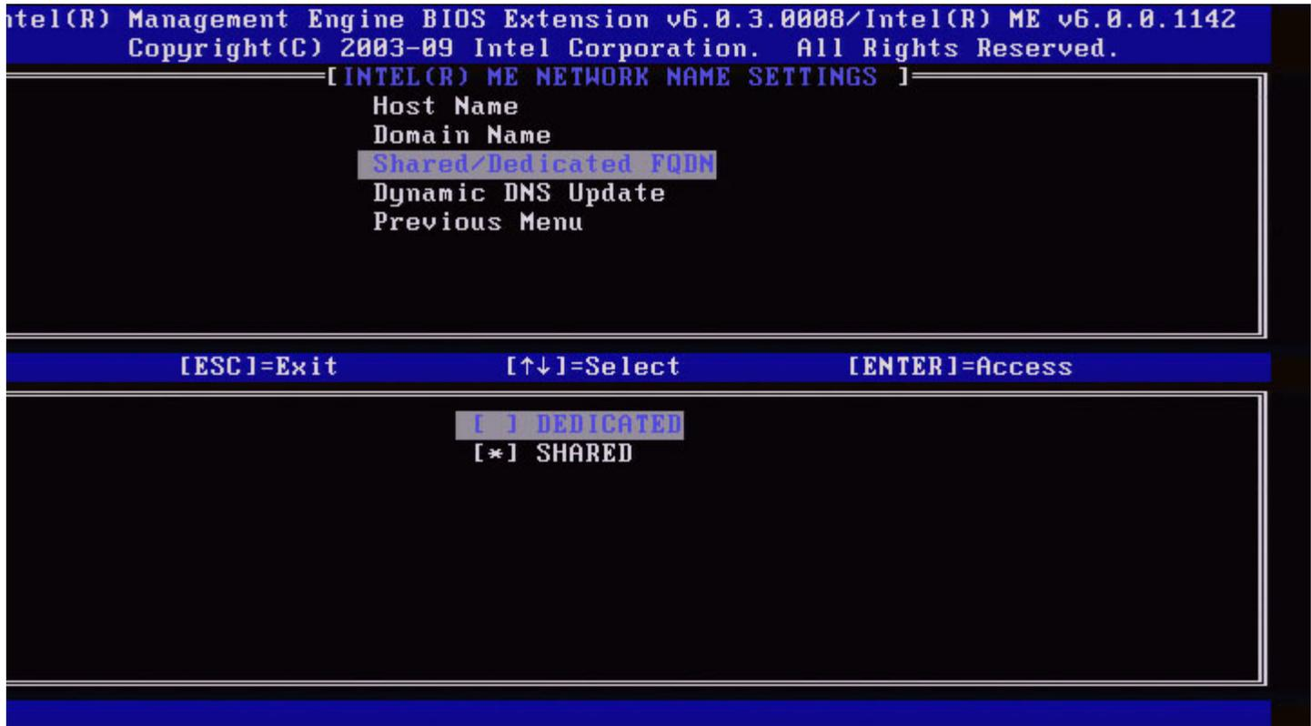
This setting determines whether the Intel ME Fully Qualified Domain Name (FQDN) (that is, the "HostName.DomainName") is shared with the host and identical to the operating system machine name or dedicated to the Intel ME.
