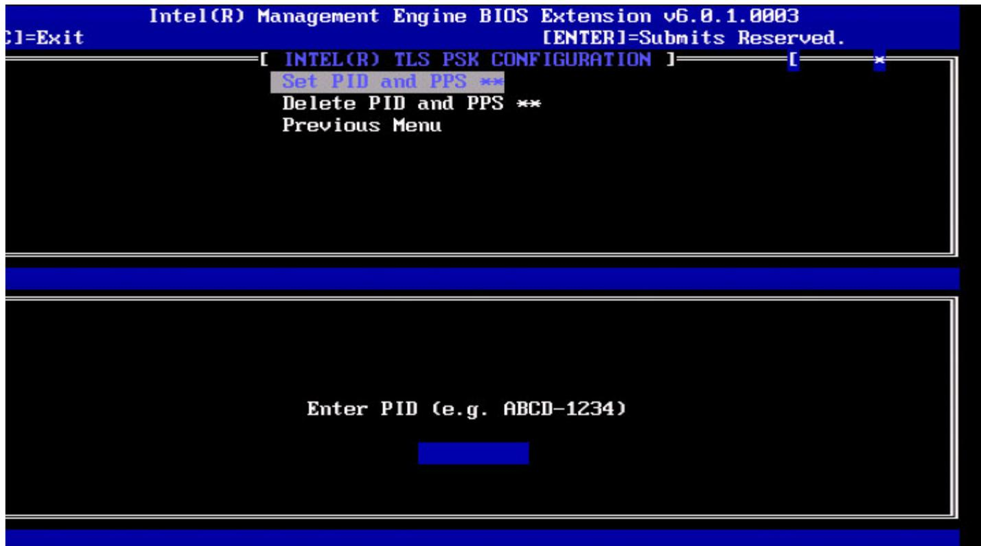
Setting the PID/PPS will cause a partial unprovision if the setup and configuration is "In-process". The PID and PPS should be entered in the dash format. (Ex. PID: 1234-ABCD ; PPS: 1234-ABCD-1234-ABCD-1234-ABCD-1234-ABCD).
